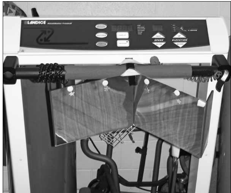
TAAP equipment: placement of 45 degree double mirror on treadmill bar.
